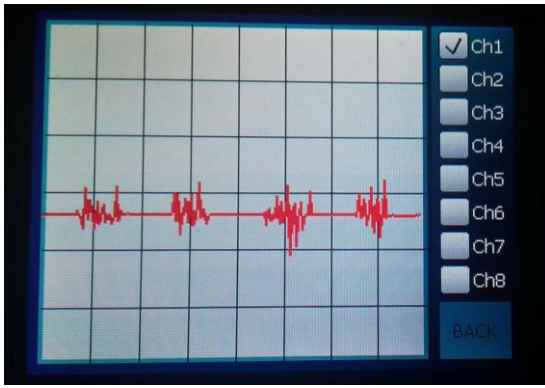
Fig. 6. EMG signal displayed in duration of 5 s with maximal display amplitude range of 10 mVpp.
