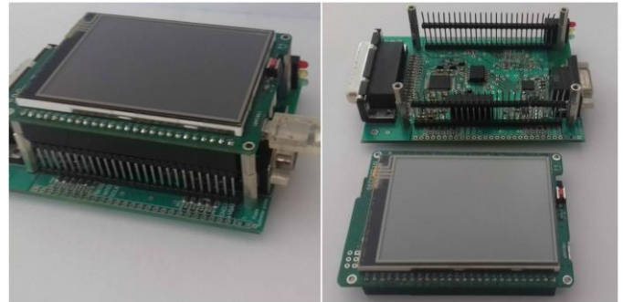
Fig. 2. The electrophysiological data acquisition system, assembled (on the left) and unfolded (on the right).
