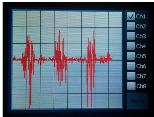
Fig. 5. Digitally filtered EMG signal displayed in duration of 5 s with maximal display amplitude range of 1 mVpp.
