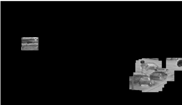
Fig. 6. Morphological image processing - dilation with square structural element
