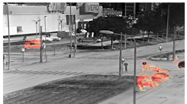
Fig 10. Motion detection and visualization – regions of interest clearly differentiated from the background
