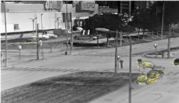
Fig. 5. Optical flow estimation based on SURF points
