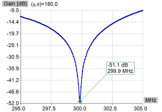
Fig. 2. Gain in backward direction in terms of frequency, obtained for  $(w_1=0, w_2=1)$
