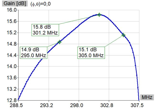
Fig. 1. Gain in forward direction in terms of frequency, obtained for  $(w_1=1, w_2=0)$
