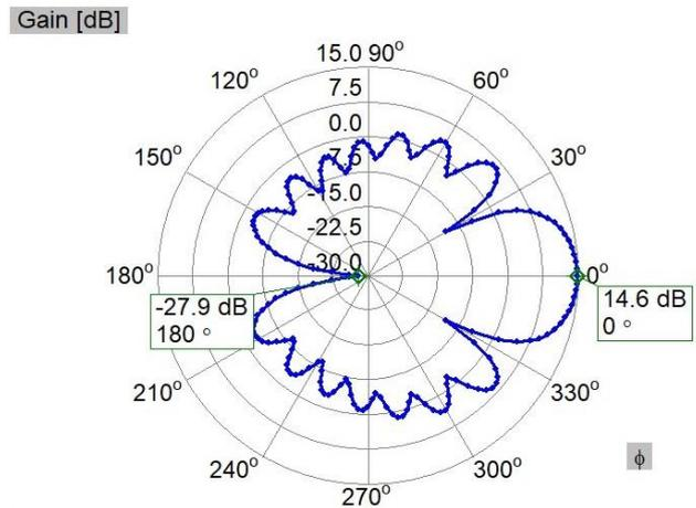
Fig. 5. Gain on 300 MHz in H-plane for one of optimal solutions
