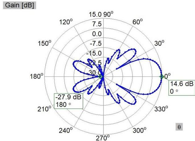
Fig. 6. Gain on 300 MHz in E-plane for one of optimal solution
