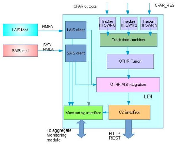
Figure 2. LDI module structure and input and output formats
