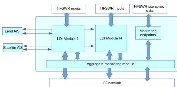
Figure 3. Structure of the central processing and monitoring process - single-process realization
