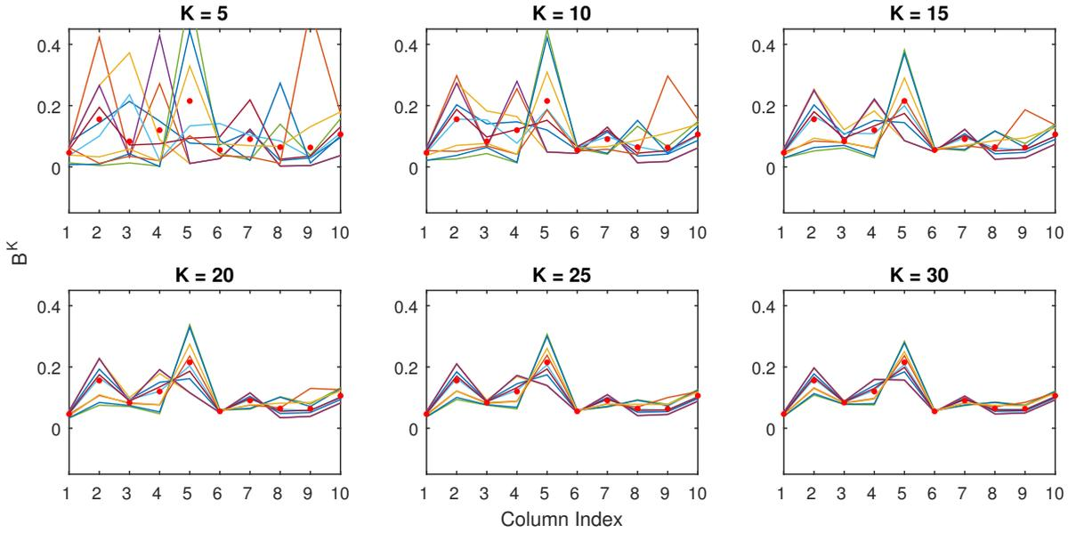
Fig. 4. Values of all rows of  $B^K$  when  $B$  is not optimized; asymptotic weights  $w$  are illustrated with red dots.
