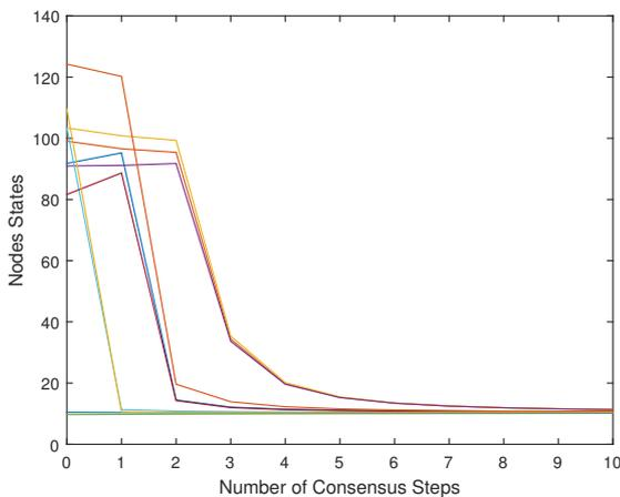
Fig. 6. Nodes' states for different number of consensus steps - non-optimized case.
