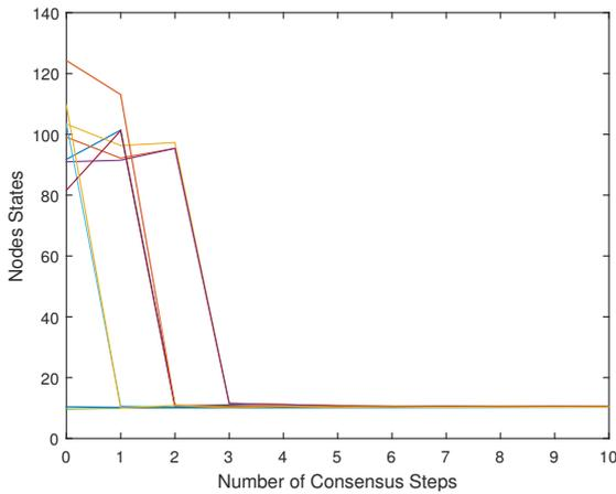
Fig. 5. Nodes' states for different number of consensus steps - optimized case.
