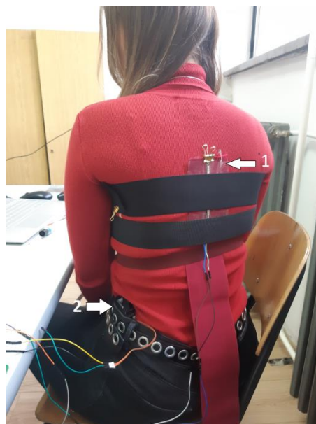
Fig. 1. Illustration of the FSR sensor and servo motor set-up
