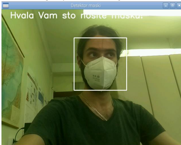
Fig. 2. Mask detection on Raspberry Pi 2B.
