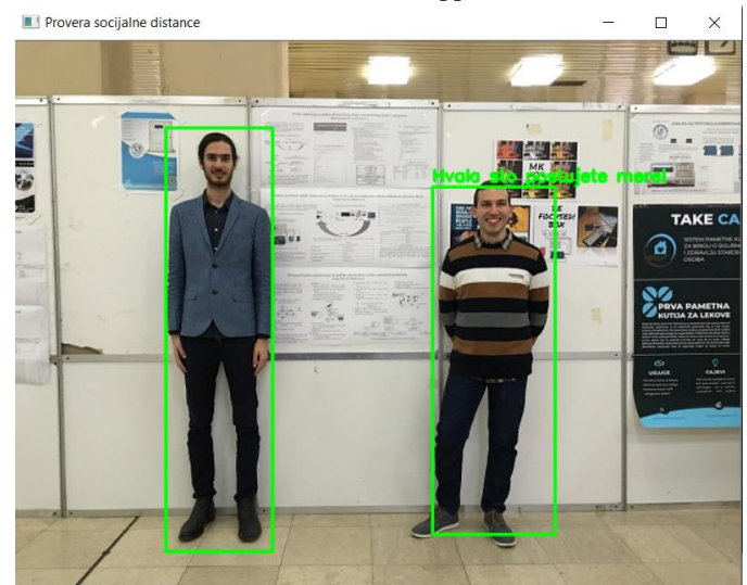
Fig. 3. The authors testing the social distancing check algorithm for threshold d =1m.
