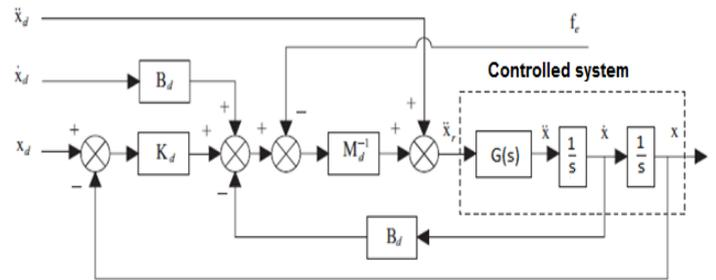
Fig. 1. The structure of a typical impedance controller.
