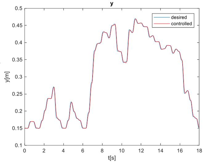
Fig. 4. y coordinate of the tool.
