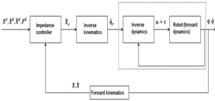
Fig. 2. Impedance control scheme used in simulation.
