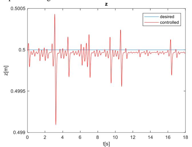
Fig. 5. z coordinate of the tool.
