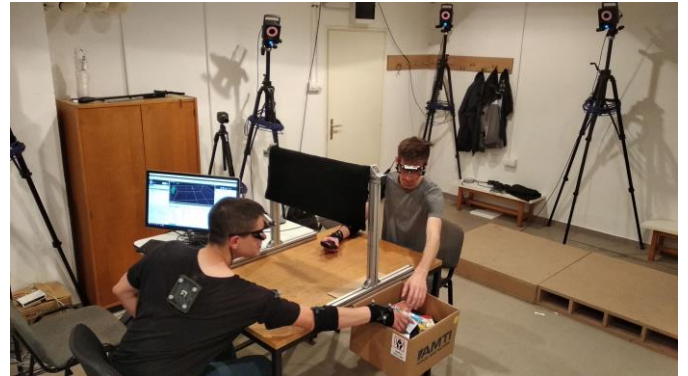
Fig. 1. Two human co-workers are picking the items from a box, scanning the barcode and handing over or placing the item on the table. During the experiment, eye gaze, head gaze, trunk, and arm motion is tracked with a Vicon motion capture system and Pupil-Lab gaze-tracking glasses.
