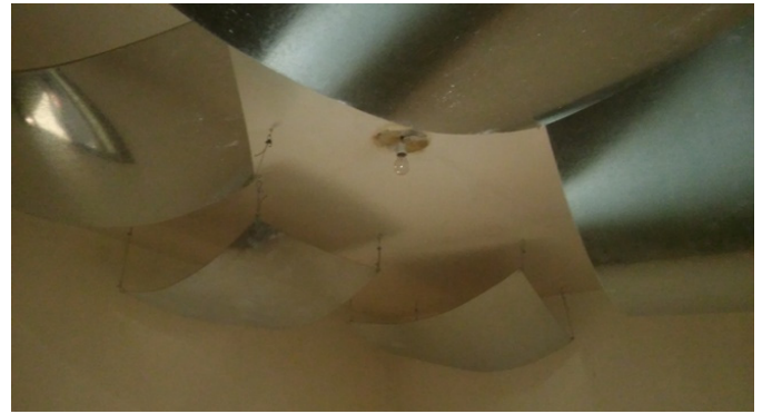
Fig. 1. Reverberation room of the Faculty of Electronic Engineering in Niš with all 5 diffusers.
