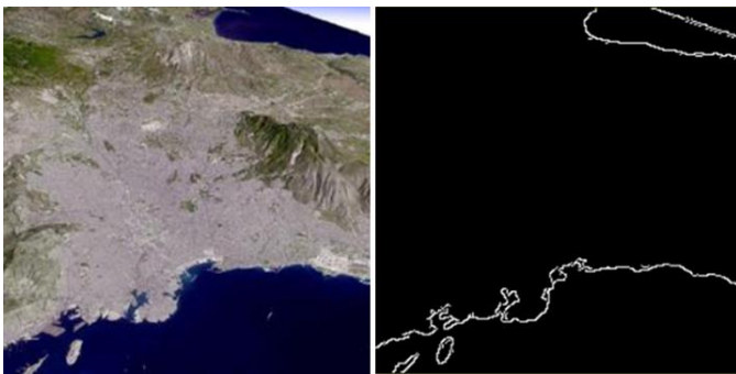
Sl.6 Atina (satelit Aster), levo - originalna slika, desno - detektovana ivica, pt=(0.420, 0.580, 0.0, 0, 255, 0, 255, 3 \times 3, 41, 213, 35, 100)
