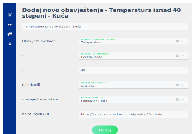
Fig. 6. Configuring an alarm for high temperature for the selected location
