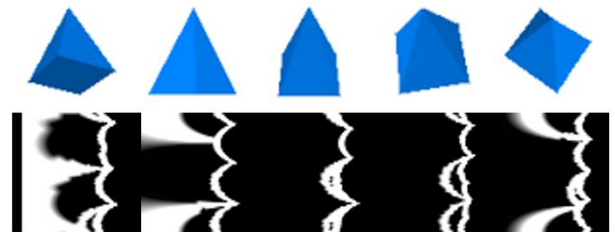
Fig. 5. Model images from multiple viewpoints (first row) and the log-polar transformations of the paired intensity images (second row)
