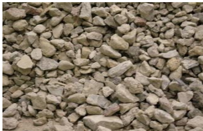
Fig. 2. Recycled Concrete Aggregates [11]
