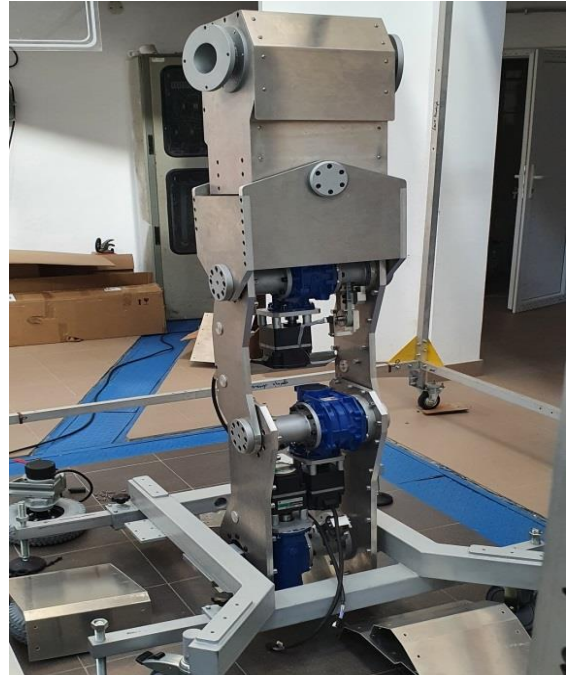
Fig. 2. The prototype of the mechanical torso of the analyzed robot.
