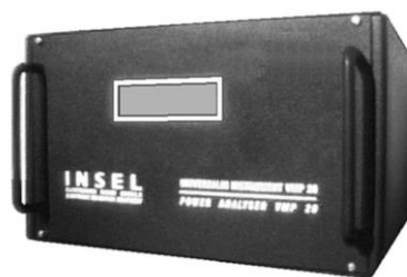
Sl. 1. Instrument VMP20 – monofazni analizator snage
