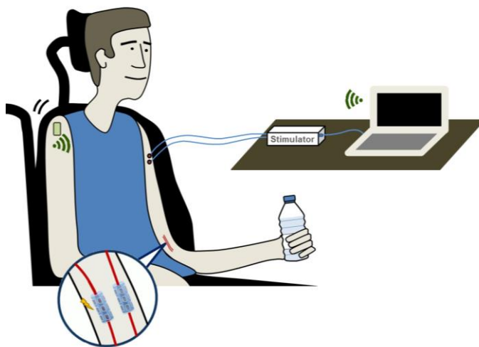
Fig. 1. AGILIS approach principle: 2 multi-contact cuff electrodes are wrapped around radial and median nerves. Percutaneous cables are connected on demand to an external pulse generator. Stimulation configuration patterns are pre-programmed to elicit hand opening/closing. The user controls contralateral shoulder movements or muscle contraction to send commands to the stimulator software: hand opening, palmar or key pinch grip...
