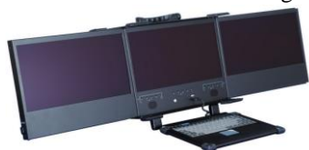
Fig. 2. Multi-sensor imaging system operator's console with three displays.
