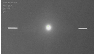
Fig. 11. Image taken with thermal imager of LRF firing in a target
