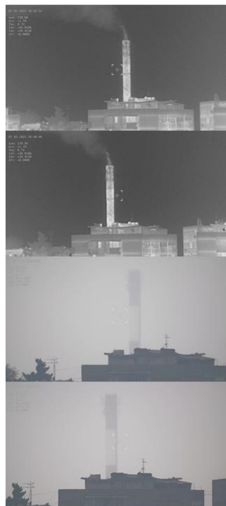
Fig. 13. A heating plant chimney at 8km distance used to verify the x-axis deviations of the reticle, in thermal and visible imager
