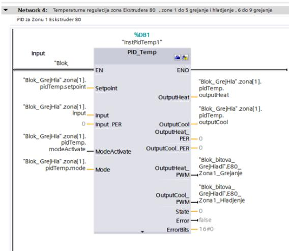
Fig. 7. Calling InstPIDTemp1 from OB30 block for zone 1
