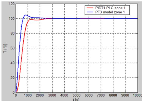
Fig. 9. Response characteristics of the calculated PID controller for PT<sub>3</sub> model and PIDT1 for Zone1 obtained by simulation using a PLC controller and a simulation library
