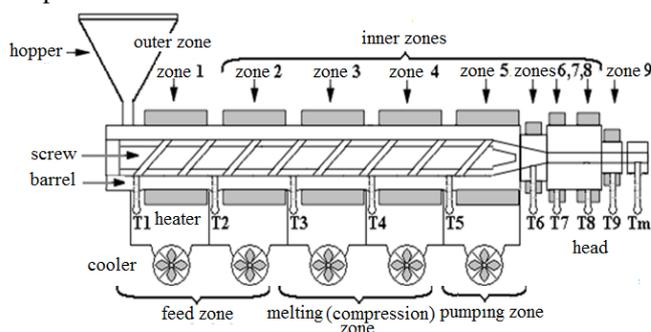
Fig. 1. Diagram of a single-screw PVC extruder
