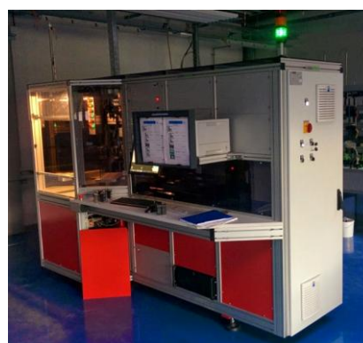
Fig. 13 Robotized system for current transformers accuracy testing in MBS factory Germany (2012.) [54]
