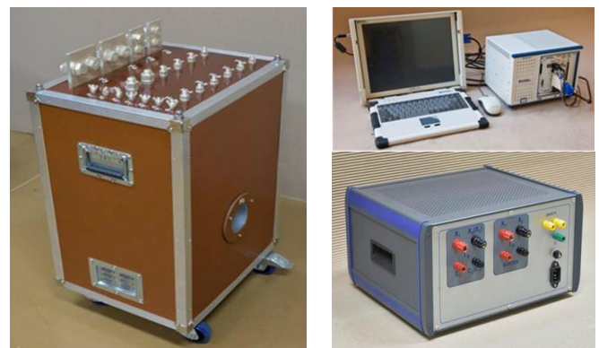
Fig. 17 Practical realization of NRC measuring system for accuracy testing of current transformer
