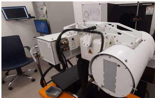
Fig. 8 A MSIS set up for rectification of visible light imager in front of the collimator
