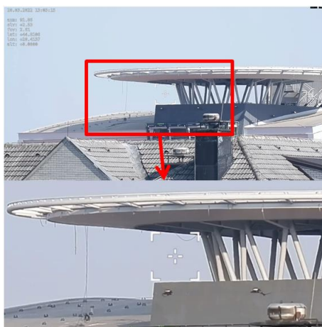
Fig. 14. A rooftop heliport structure with upper and lower limits, at the 620m distance, used to verify the y-axis
