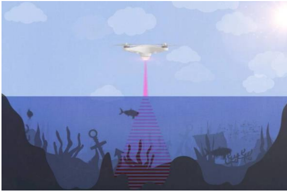
Fig. 11. An illustration of Stanford's photoacoustic airborne sonar system [3]
