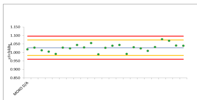
Fig. 2. Unified Sheward chart for 4 MOKO 100 type of ambient dose equivalent rate monitors
