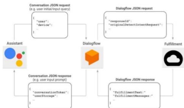
Fig. 1. The diagram shows the path that requests go from Assistant through the Dialogflow till the Fulfillment and response traveling back to the Assistant.
