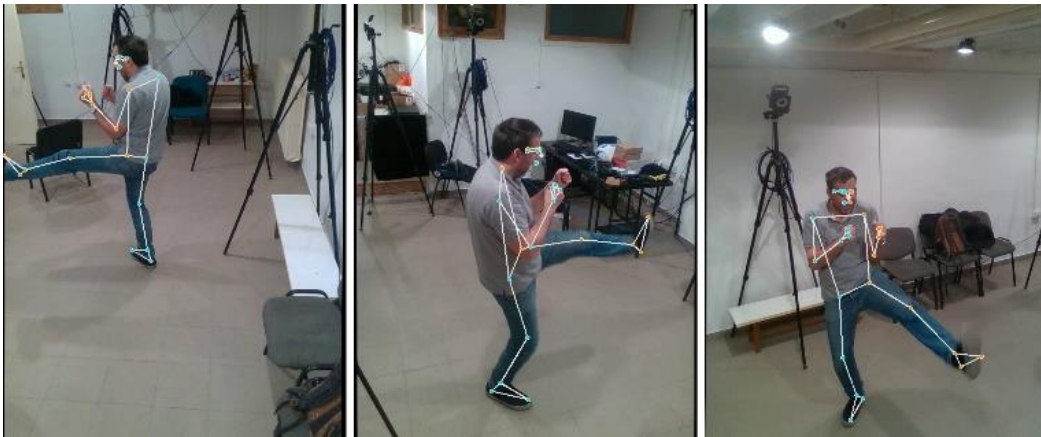
Fig 6. A frame from all 3 cameras taken at the same time with detected keypoints drawn over
