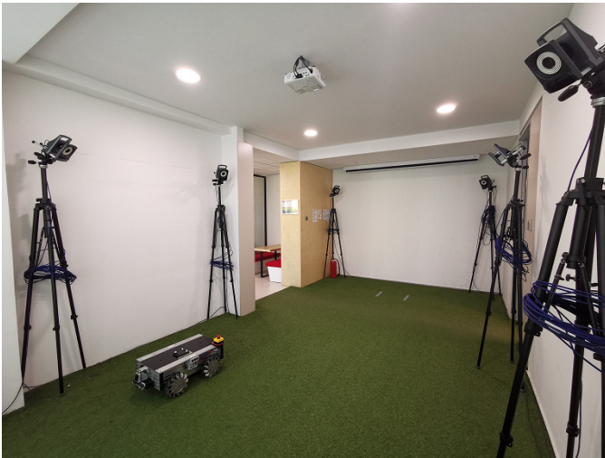
Fig. 1: Experimental setup with Vicon cameras and mobile robot
