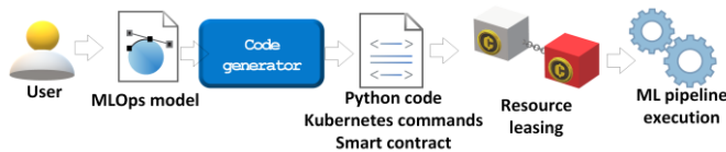
Fig. 4. Blockchain-enabled model-driven MLOps workflow.
