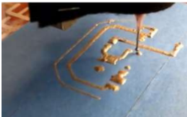
Fig. 3. Results after applying the 3D printing method with using the golden wire in production of one circuit board: a) correct and b) incorrect
