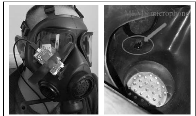
Fig. 2. MEMS microphone board attached to the gas mask (left figure), where microphone is inserted in the mask interior (right figure)
