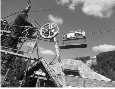
Fig. 12, In-situ MRT configuration, ski-lift
