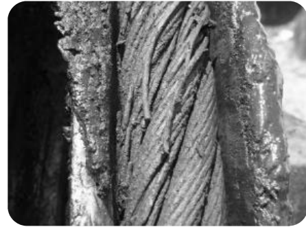
Fig.1/a Critical condition of a 1-meter rope segment
