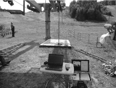
Fig. 14, Typical in-situ MRT inspection
