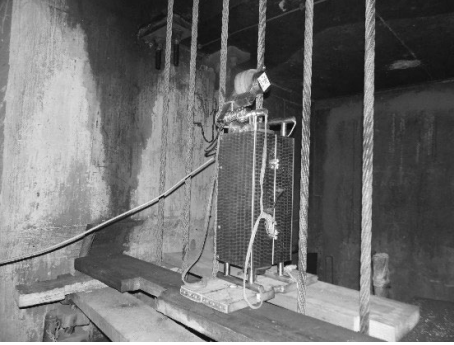
Fig. 13, In-situ MRT of multi-rope mine hoist
