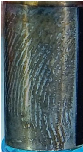
Fig.6. Development of a fingerprint on the brass cartridge case by the electrodeposition of nickel with the 30 mA/cm 2 current density and a deposition time of 10s, after photo editing (the reflection from the surface that occurred during photography is reduced).
