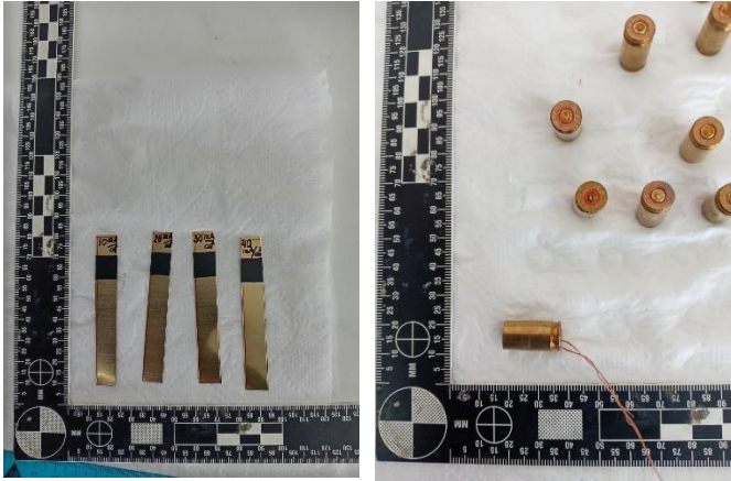
Fig.1. Brass samples to determine the rate of nickel electrodeposition (left) and samples of brass cartridge cases after cleaning, without fingermarks (right)
