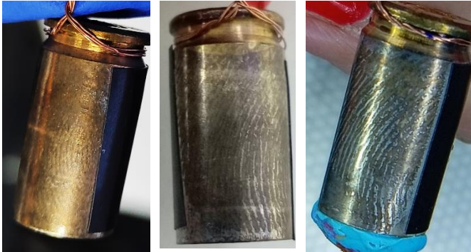
Fig.5. Development of fingerprints on the brass cartridge cases by the electrodeposition of nickel with the 30 mA/cm 2 current density and a deposition time of 5s (left), 7s (center), and 10s (right).
