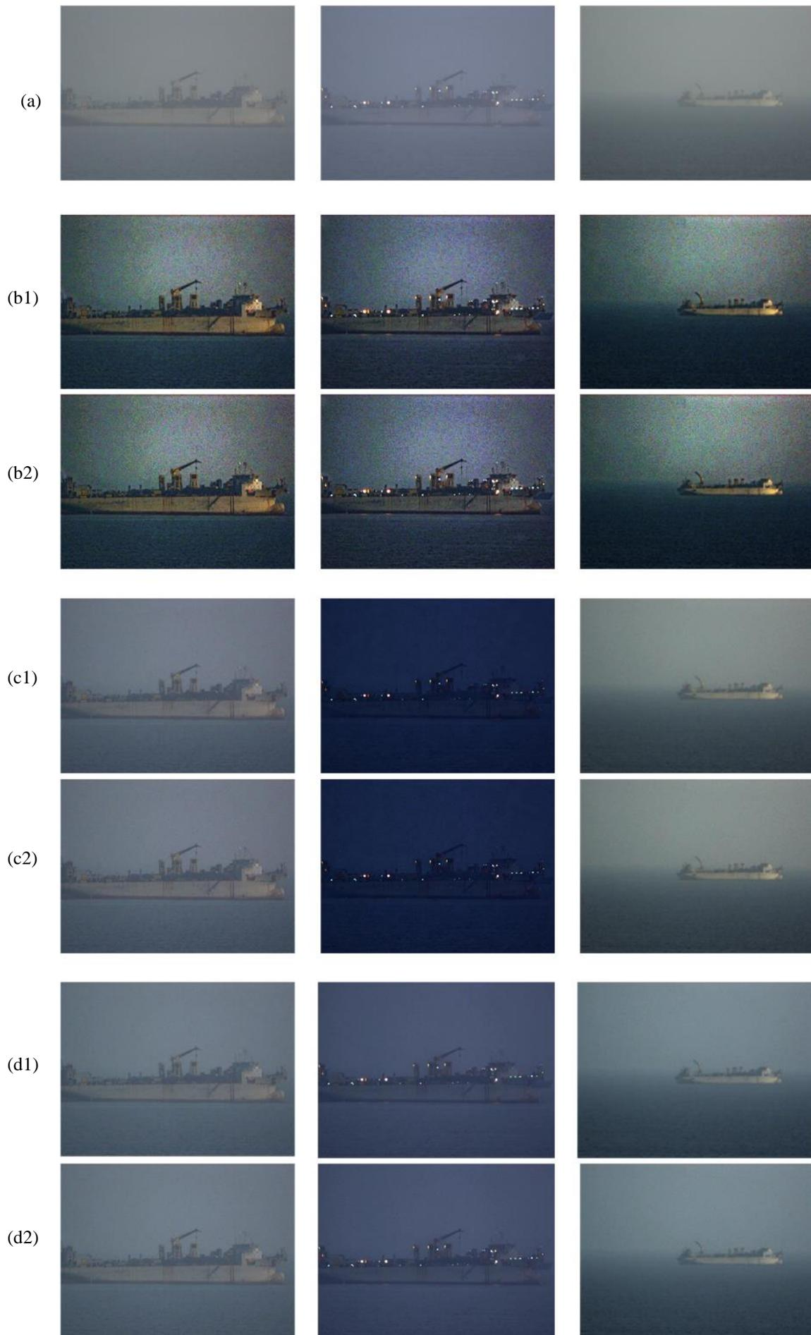
Fig. 5 Image dehazing and unsharp-mask: (a) original image, (b1) DCP, (b2) DCP&unsharp-mask, (c1) CAP, (c2) CAP&unsharp-mask, (d1) DNET, (d2) DNET&unsharp-mask
