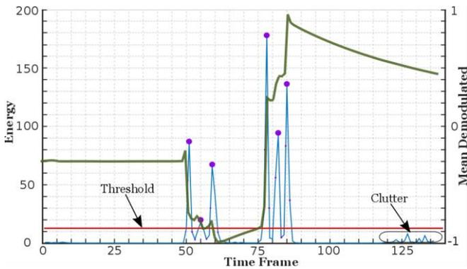
Fig. 4. Extracted signal energy diagram with marked maximum points
