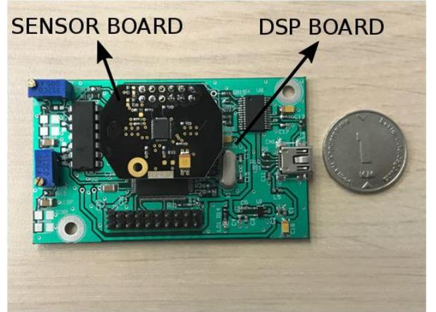
Fig. 2. Integrated sensing/DSP solution
