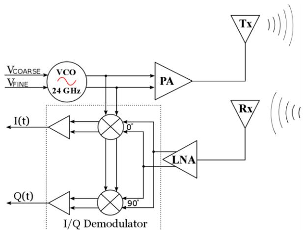
Fig. 1. Block diagram of quadrature Doppler radar measurement system
