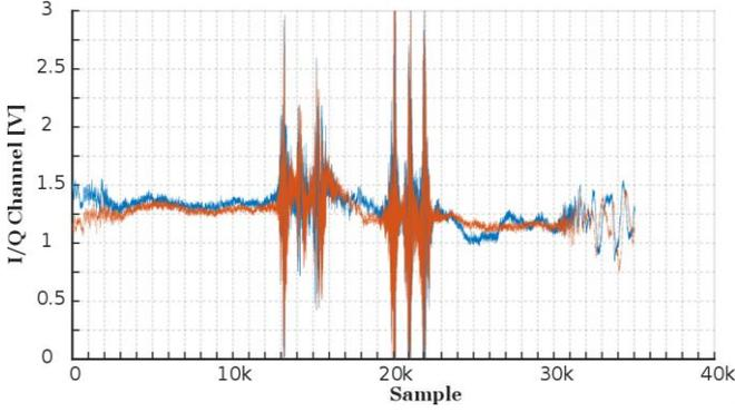
Fig. 3. I/Q signals for three different persons passing through the door
