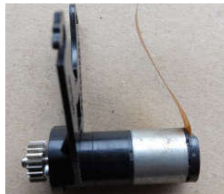
Fig. 1. Motor Faulhaber 1516.A0210 with planetary gearhead and magnetic incremental encoder
