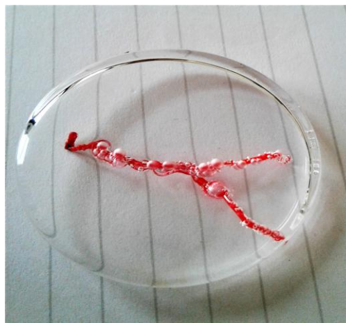
Figure 6. Distorted red ABS microstructure with residues of acetone after 5min at the temperature of 100°C in oven.
