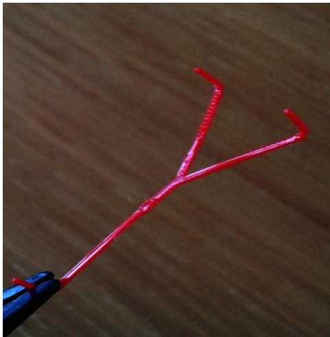
Figure 1. Example of red ABS bifurcated microstructure.
