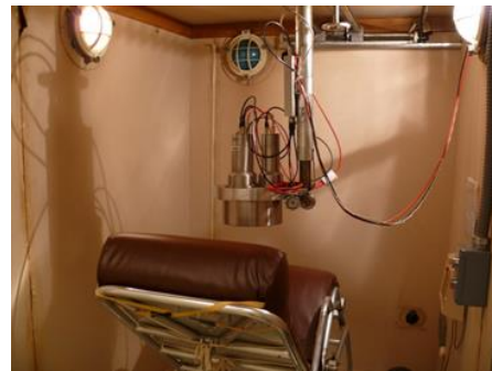
Fig. 3. WBC NaI(Tl) scintillating detector in steel protective chamber.
