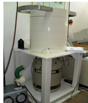
Fig. 4. Gamma spectrometry ORTEC GEM 50 system.
