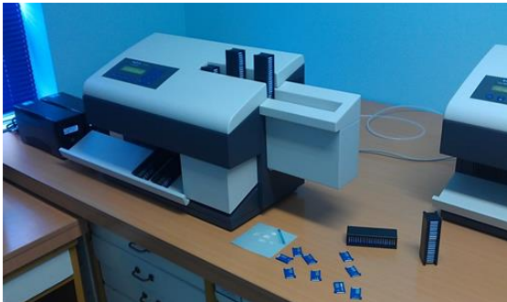
Fig. 2. Thermo-luminescent dosimeters RADOS reader type RE-2000.
