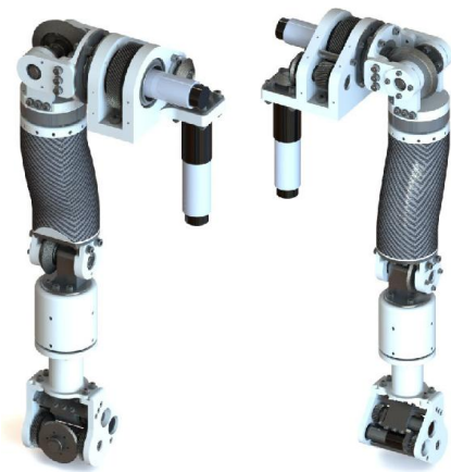
Fig. 7. The right arm with 7 DOFs – front and back view
