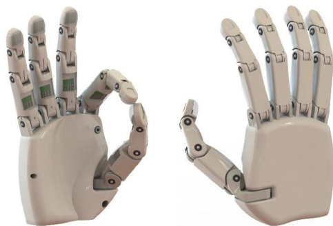
Fig. 8. The underactuated hand with 5 DOFs and total 16 joints
