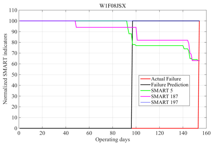
Fig. 3. Example of failure prediction for drive with serial number W1F08JSX
